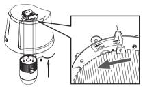
7. Connect the circuit board to the connector of the Speed Dome Camera as shown in the figure.
